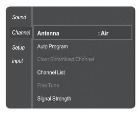
3 Press ▲ or ▼ to highlight **Fine Tune**, then press **ENTER** to access the *Fine Tune* screen.
